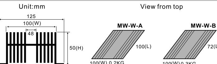
MW-W-A: Compatible with Single Phase SSR with load at 40A(72\*100\*50)
