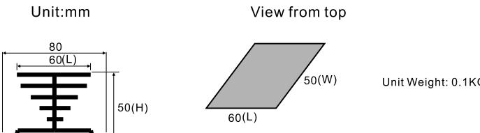
MW-I: Compatible with Single Phase SSR with load at 10A and 25A(60\*50\*50)
