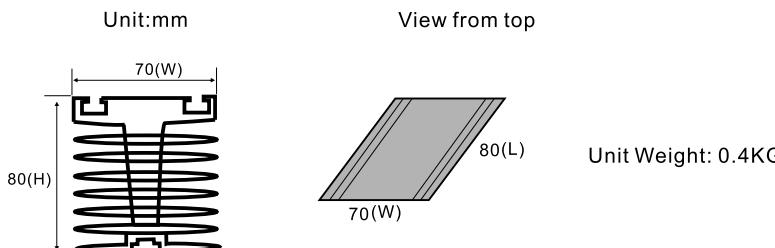
Compatible SSR: Single Phase SSR with load at 80A/100A/120A.(80\*70\*80)
